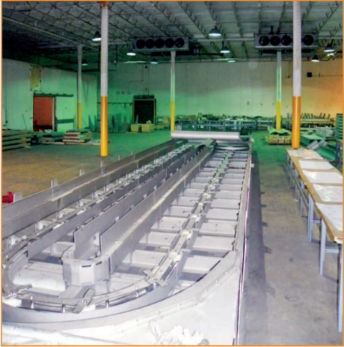
The MultiDisc® Screens (MDS) are preassembled at a nearby staging location and measure 53 feet by 11 feet. Photos/Site
