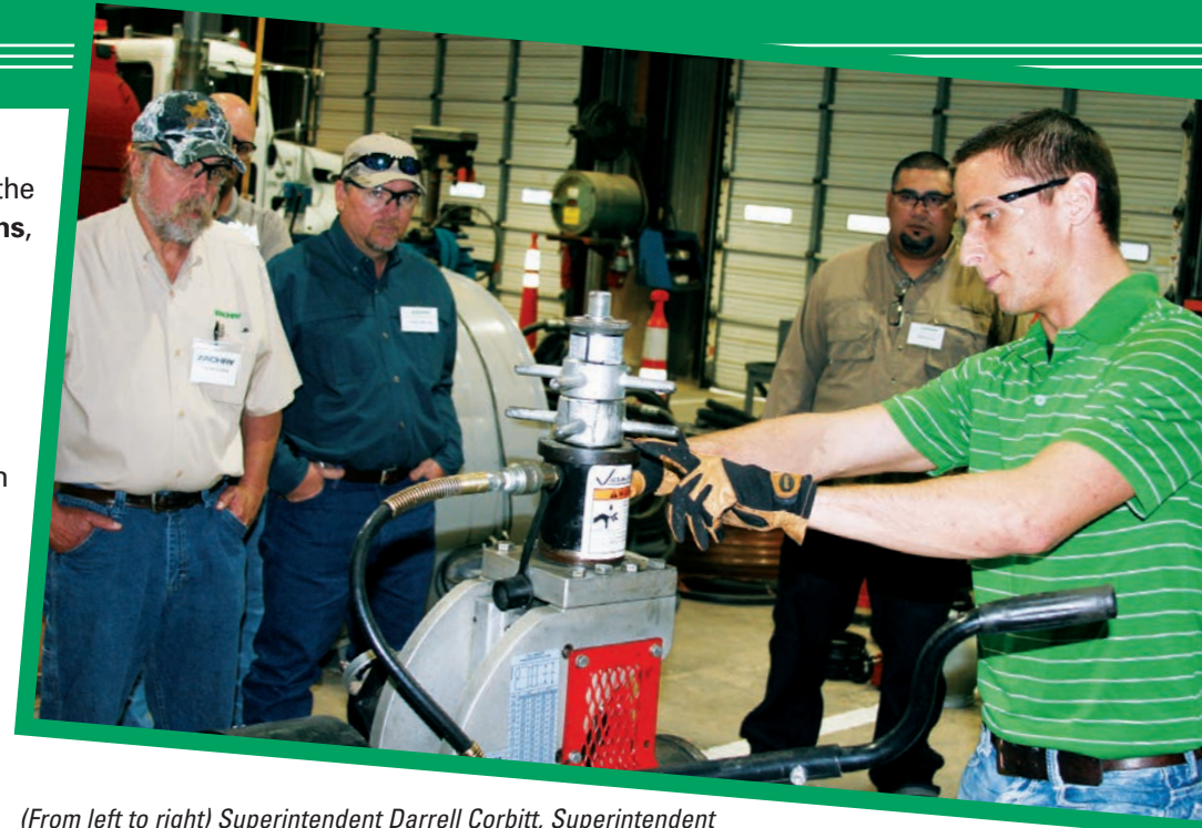
(From left to right) Superintendent Darrell Corbitt, Superintendent Scotty McCain and General Foreman John Garcia watch as a vendor demonstrates a device that grooves pipe to form victaulic connections. Photo/Doug House
